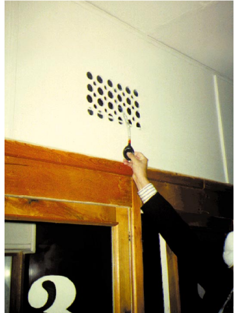
Using a smoke tube to monitor air flow in sputum collection booth at a TB facility in Riga, Latvia
